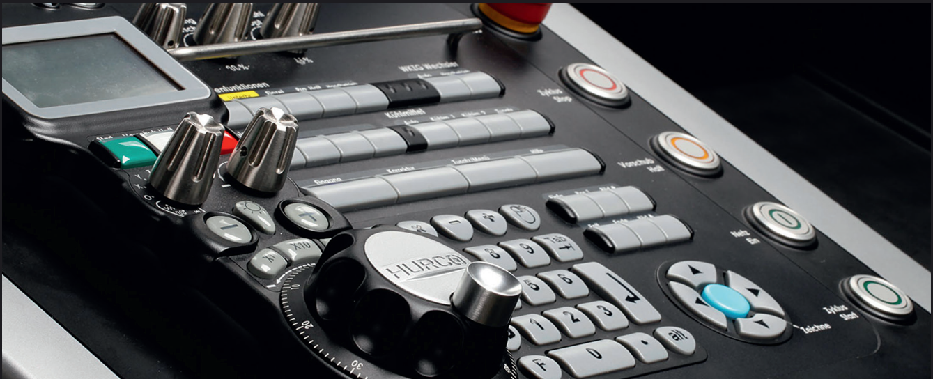
HURCO MAX® 5 CNC control system with electronic handwheel.
